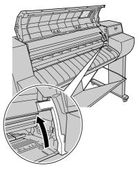
**3** If the jammed sheet is visible, grip the sheet by the left and right sides and pull it toward you out of the printer.
